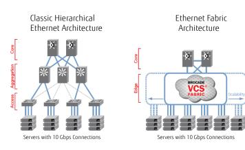
**Figure 1:** Compared to classic Ethernet architectures, Ethernet fabrics allow all paths to be active and provide greater scalability—while reducing management complexity.
