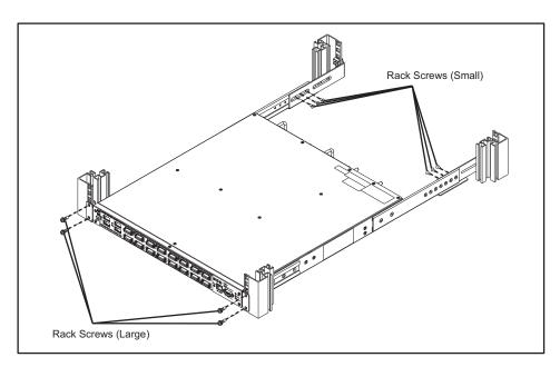
2. Slide the XG2000C forward, and remove it from the rack.
