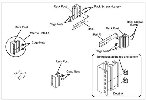
[When the rack has round post holes (top of view)]
