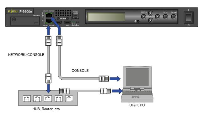
Figure Connection to a network
