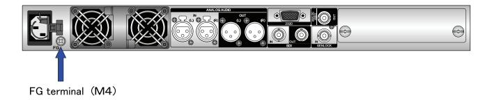
Figure Connection to ground
