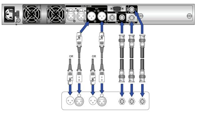
Figure Audio and video input device connections
