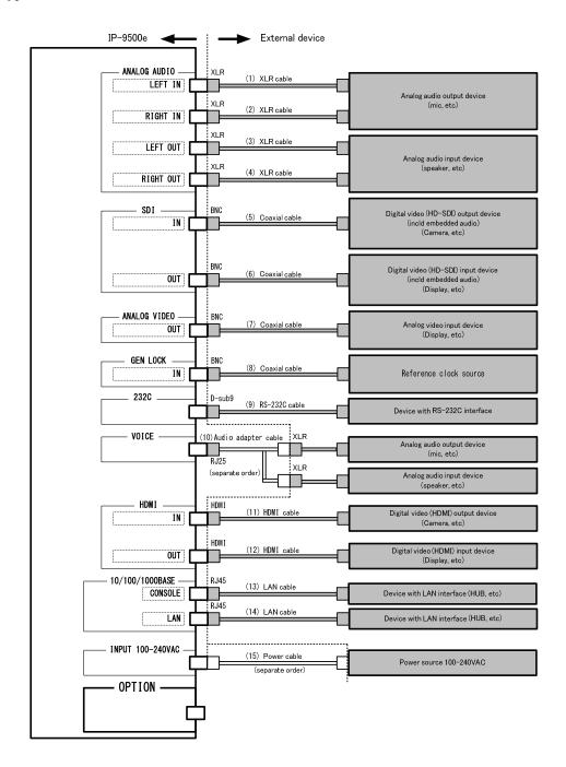
When constructing a system that uses IP-9500e, consideration must be given so that its boundary between IP-9500e and other devices is similar to that shown in the above figure. Since the type of work may change depending on the system, procure equipment and perform work based on consultations with a system designer.
