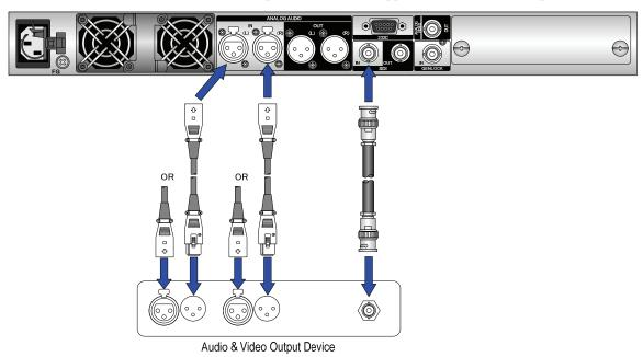
Figure Audio and video output device connections
