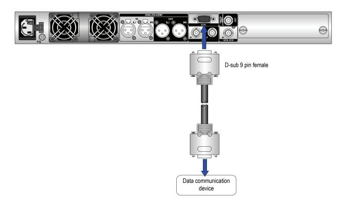
Figure Connection to RS-232C input/output device
