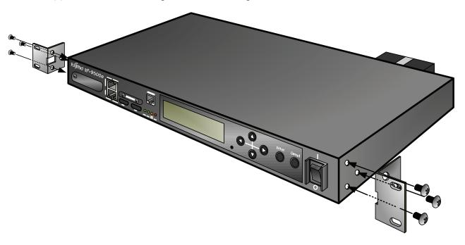
(4) Install IP-9500e on 19" rack using the four pan screws (M5) attached.
