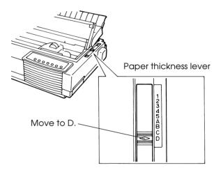
Adjusting the paper thickness lever
