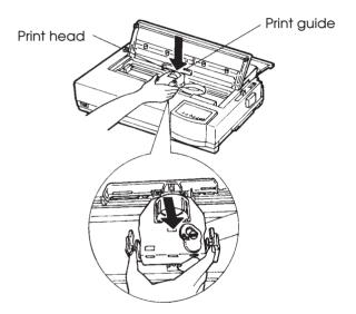
Installing the new ribbon cartridge
