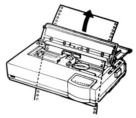
Passing continuous forms paper from under the printer
