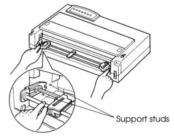
Removing the tractor unit
