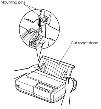
Installing the cut sheet stand
