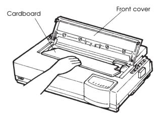
Removing the shipping restraint cardboard
