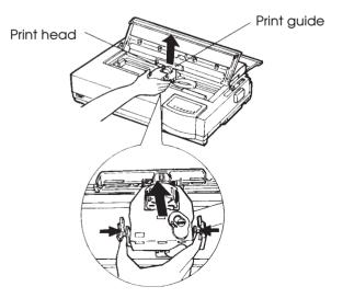
Removing the ribbon cartridge
