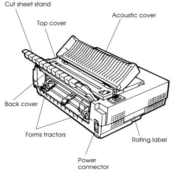
Looking at the printer from the back with the cut sheet stand and back cover removed, you can see the following parts of the printer:
