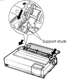
Installing the tractor unit for pull-tractor feed
