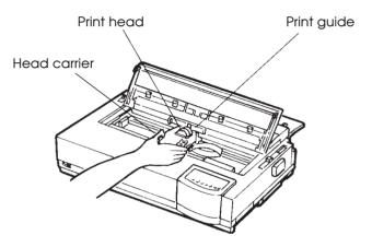
Installing the ribbon cartridge
