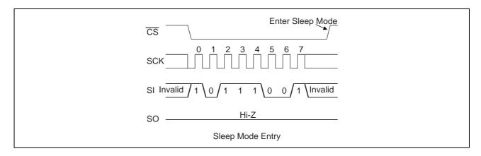
Returning to an normal operation from the SLEEP mode is carried out after  $t_{REC}$  (Max 400  $\mu$ s) time from the falling edge of  $\overline{CS}$  (see the figure below). It is possible to return  $\overline{CS}$  to H level before  $t_{REC}$  time. However, it is prohibited to bring down  $\overline{CS}$  to L level again during  $t_{REC}$  period.
