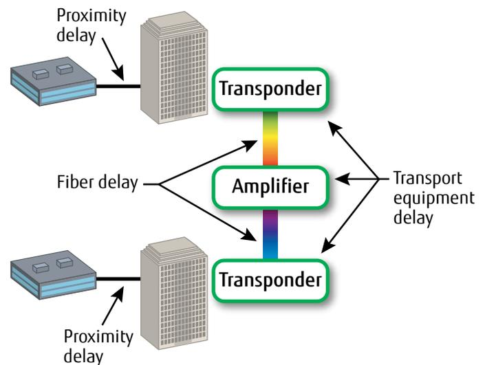
Figure 1: Sources of latency in optical transport networks
