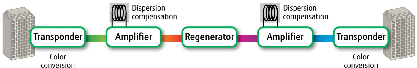
Figure 2: Optical networking functions that can increase latency
