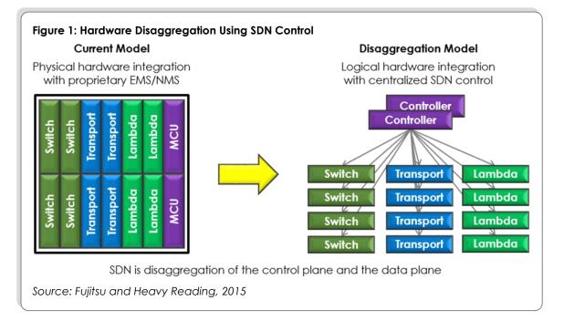
To be clear, little is accomplished under the SDN-controlled hardware disaggregation model if the SDN control protocols and network management systems remain proprietary and closed. For this reason, tremendous attention is being paid to defining standards around SDN control and network management in SDN-based networks.
