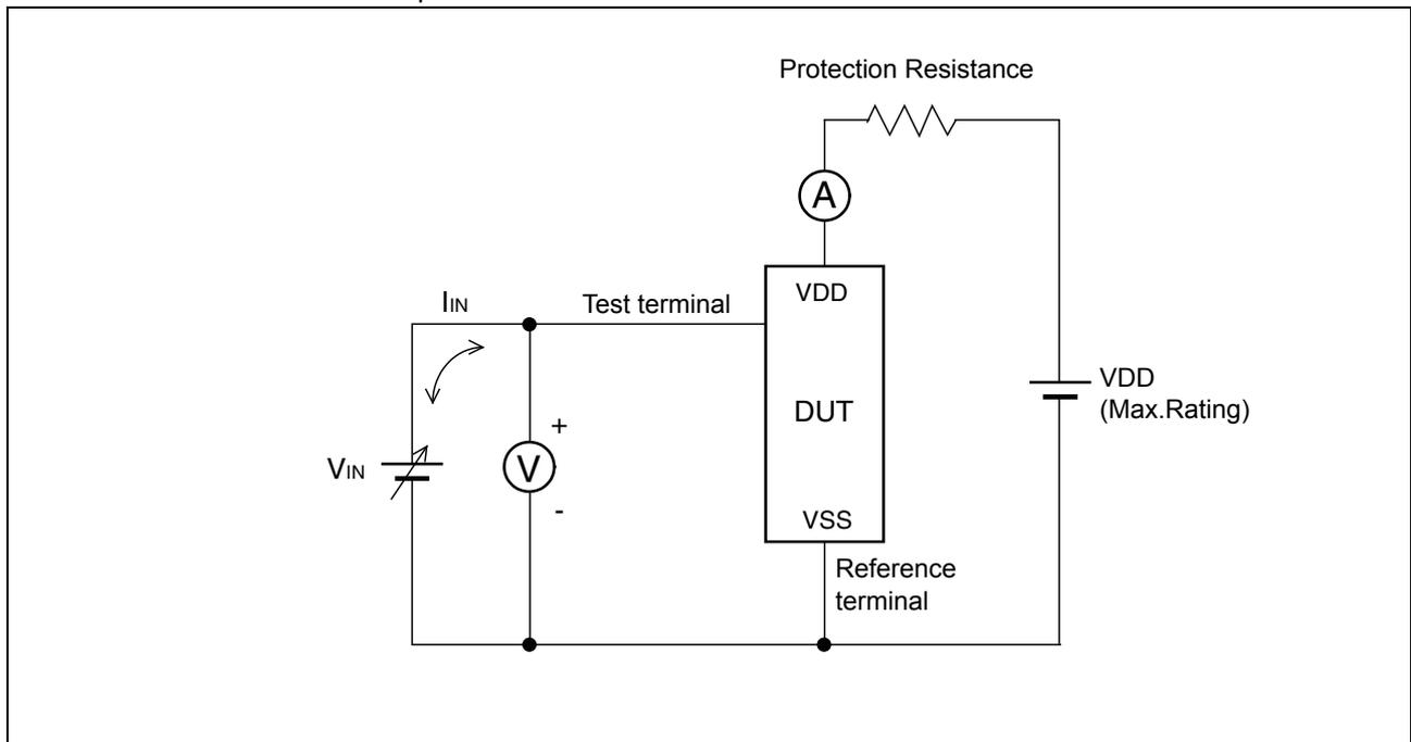
Note : The voltage  $V_{IN}$  is increased gradually and the current  $I_{IN}$  of 300 mA at maximum shall flow. Confirm the latch up does not occur under  $I_{IN} = \pm 300 \text{ mA}$ .
