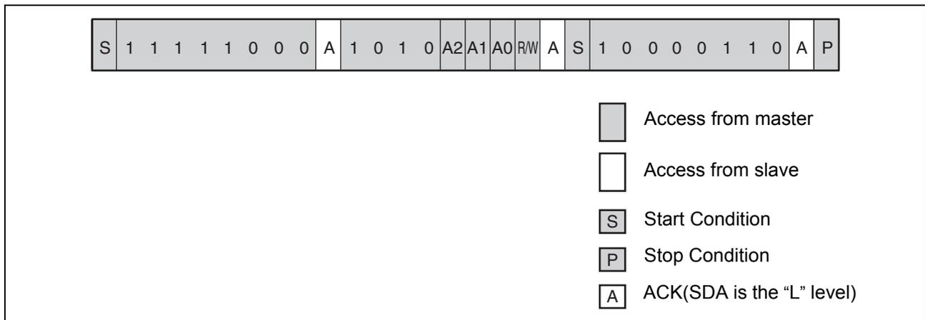
Even if the MB85RC64TA stays in the Sleep mode, SDA and SCL signals are monitored. Following sequences enable the transition to Standby mode after recovery time ( $t_{REC}$ ) of internal regulator circuits.
