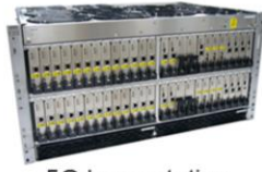
5G base station control equipment
