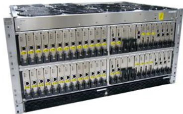
5G base station control equipment
